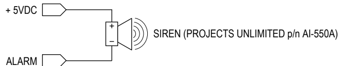
FIGURE 7. Using a siren to make the ALARM output audible.
